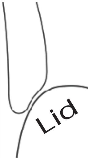
**Lid Rest Technology at Work.** Creating uniform edge profile lets the lens rest on the lid, creating an evenly distributed "cushion" for the lower lid and allows for proper lens translation in downward gaze.
